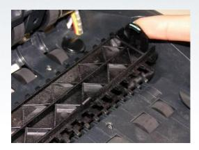
• Hold the CIS support to clean the camera lens.
