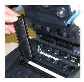
• Remove any debris and dust. Clean the Contact Image Sensors with a soft, lint-free cloth dampened with Isopropyl Alcohol or with eye glass cleaner.
