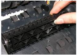
• Open the rear CIS support by pressing the right tab in and lifting up.
